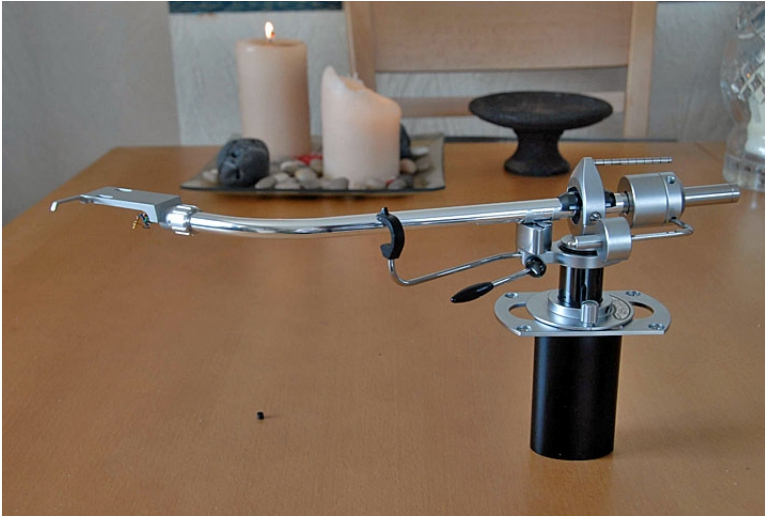
Photo 11 and Photo 12 – Tonearm cueing mechanism set for correct up and down movement.
